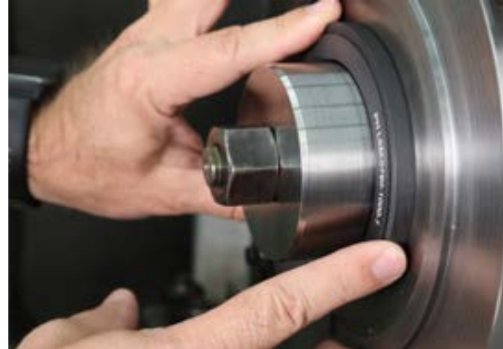
Installing the Seal
