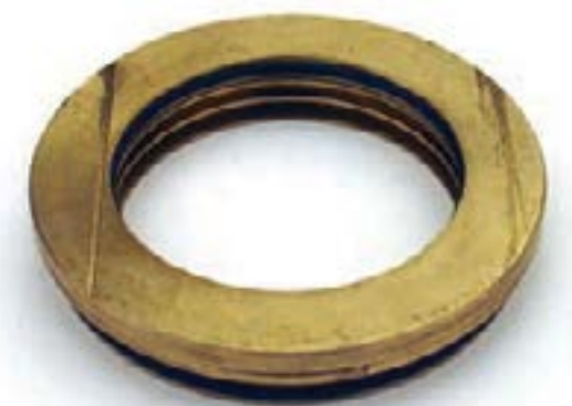
Failed seal resulting from improper installation
