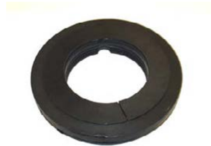
Failed seal resulting from improper fit
