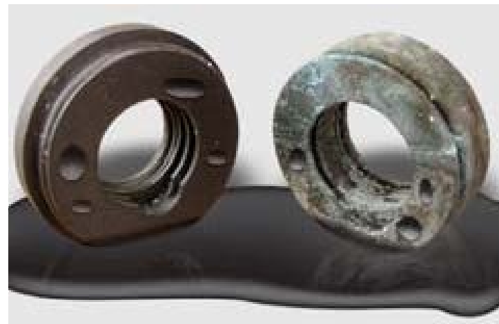
PTFE vs. metal after sulfuric acid soak
